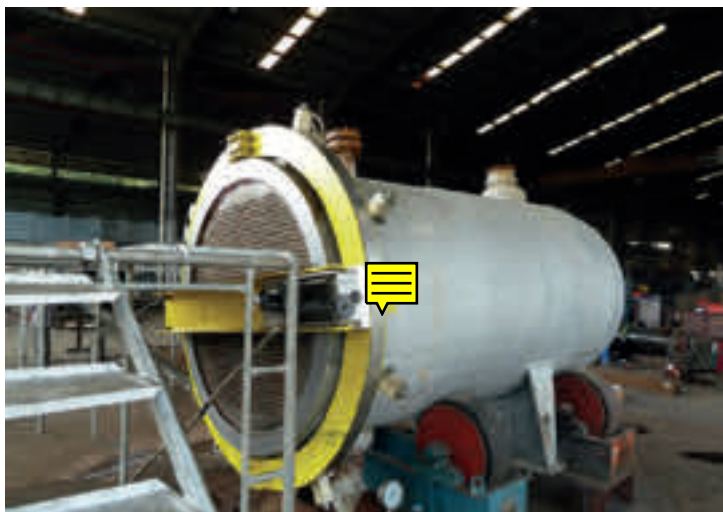
Figure 4. General view of E-02A tubesheet cross section after cutting at CS02.
