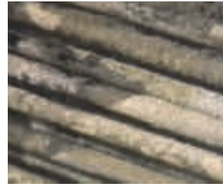
Figure 4. Under deposit corrosion.
