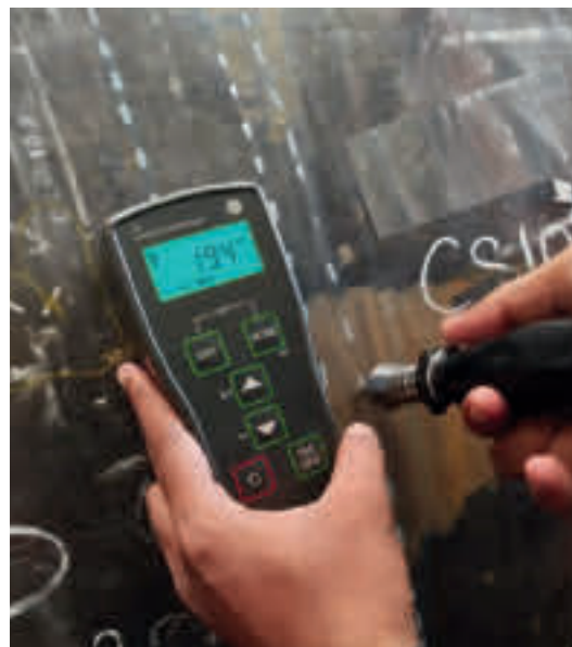
Figure 7. Hardness testing was performed pre and post heat treatment.
